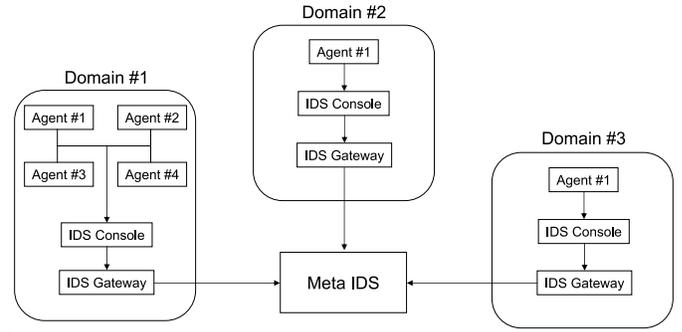
Fig. 1. General setup of the IWS and underlying IT security tools
